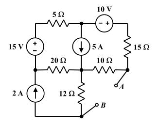
Find the Thévenin equivalent circuit with respect to terminals A and B.
